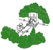
WE NEED ROOM TO WORK SAFELY ON THIS DEVICE. PLEASE KEEP SHRUBS AND STRUCTURES 10 FEET AWAY FROM THE FRONT WITH LOCK AND ONE FOOT FROM THE OTHER THREE SIDES. OBSTRUCTIONS MAY BE DAMAGED OR REMOVED DURING SERVICE RESTORATION OR MAINTENANCE.
