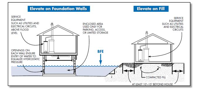
(2) Elevation on a crawl space, stilts, piles, walls, etc.
